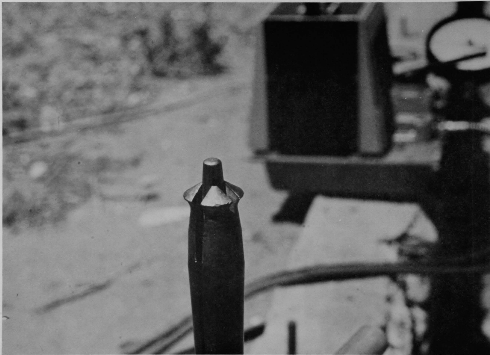
FIGURE 20. Expanding Bit Used in Concrete Spalling Technique
